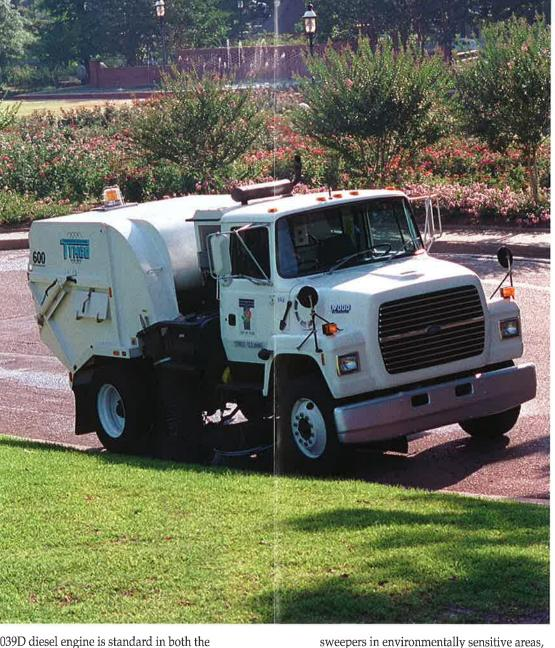
4039D diesel engine is standard in both the 4.75-cubic-yard-capacity (3.61-m³ capacity) Model 350, as well as Tymco's larger and most-popular sweeper, the 7.3-cubic-yard (5.5-m³) Model 600. The John Deere 4039T is also available on the Model 600, depending on the altitude and working environment of the sweeper.
